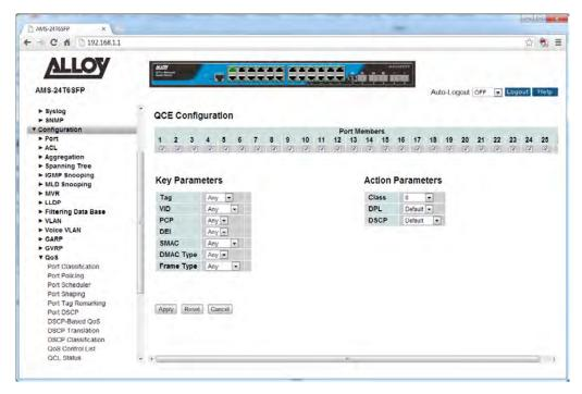
Fig. 108 Adding a QoS Control List Entry
