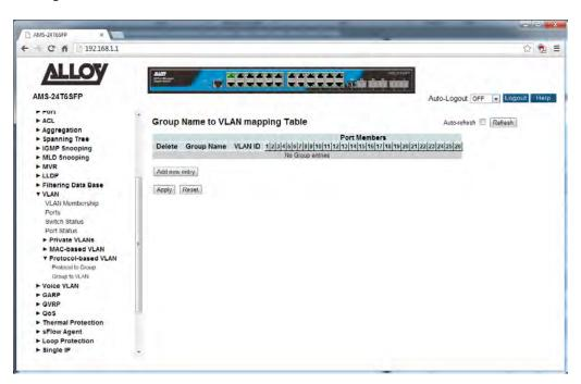
Fig. 84 Group to VLAN Mapping
