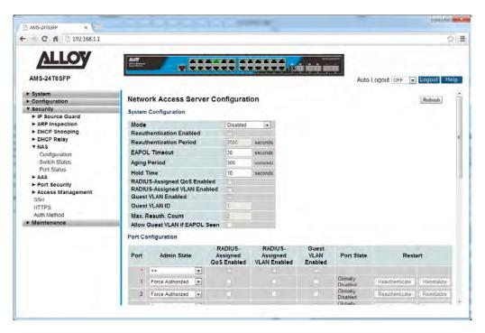
Fig. 134 Network Access Server Configuration
