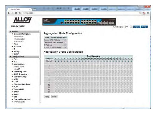
Fig. 32 Configuring a static trunk group
