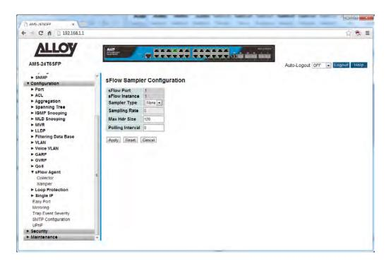
Fig. 114 s-Flow Agent Sampler Port Settings
