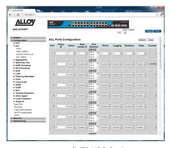
Fig. 27 Port ACL Configuration
