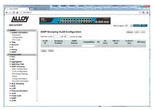
Fig. 48 IGMP VLAN Configuration
