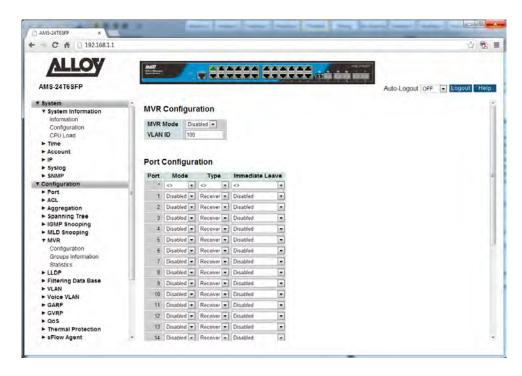
Fig. 59 MVR Configuration
