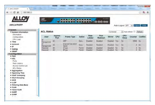
Fig. 31 Viewing the Access Control List Rules
