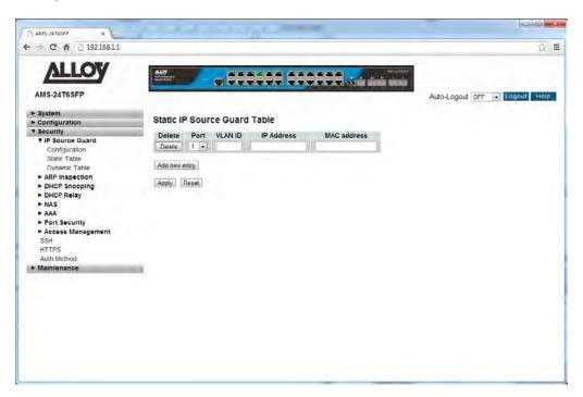
Fig. 125 Static Table Configuration
