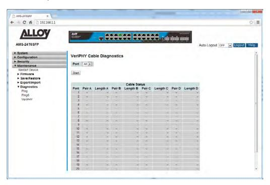
Fig. 159 VeriPHY Cable Diagnostic Test
