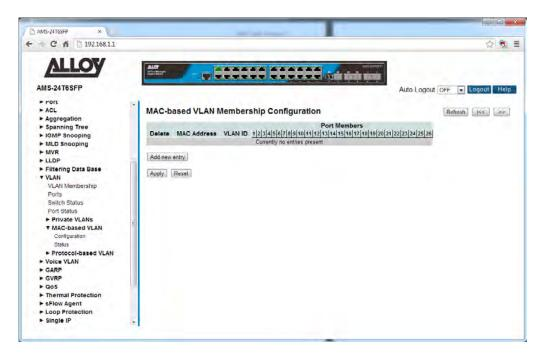
Fig. 81 MAC-based VLAN Configuration
