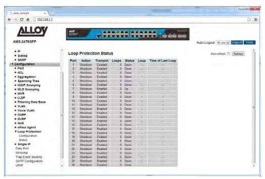
Fig. 116 Loop Protection Status
