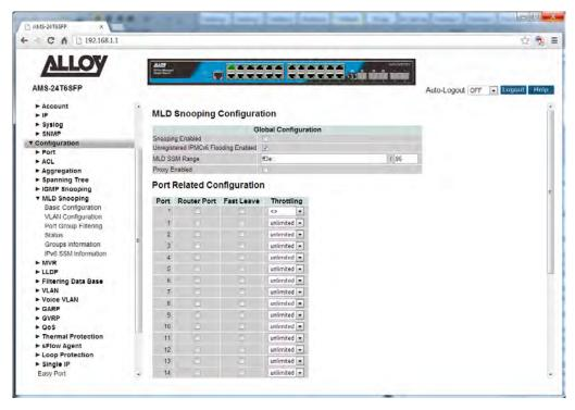
Fig. 53 MLD Snooping Configuration
