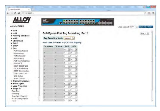
Fig. 102 Port Tag Remarking – Mapped Mode
